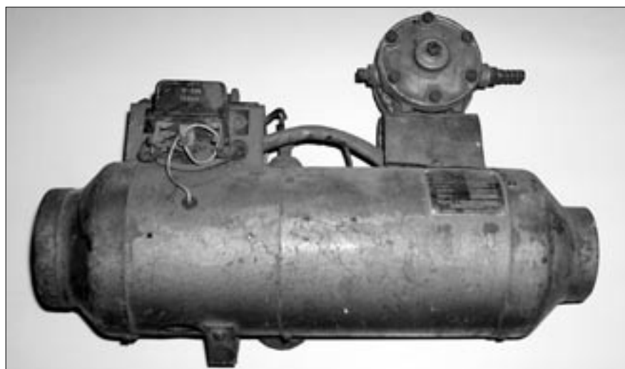
The Eberspächer independent heater from the Tatra 805 of Hanzelka. The production year 1958/59 is marked on the product plate. It is drawing no. 8516, production number 2006 or 2000 (the last numeral is not clear)
